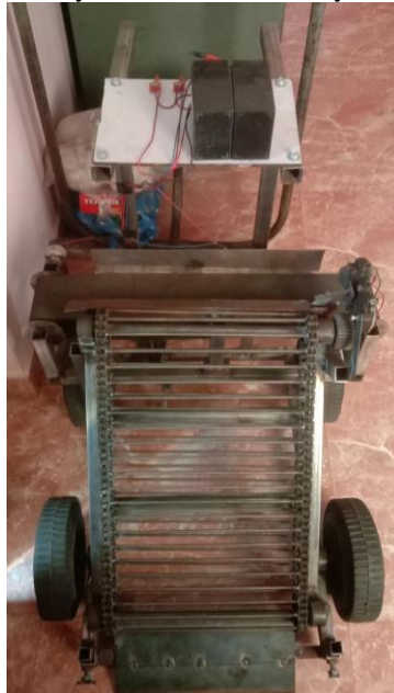
Figure 6: Developed onion harvester
